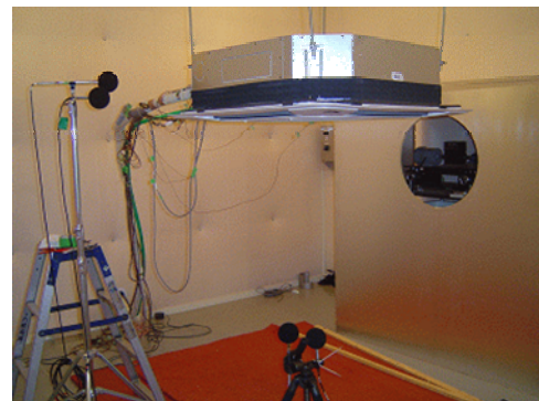
(c) Semi anechoic chamber and indoor unit
